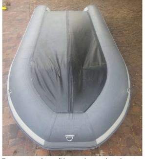
• Transoms tend to pull loose when outboard motors are left hanging on them, this phenomena is exacerbated, when the boat lies unattended in direct sunlight. Pontoon-to-transom turnbuckle brackets will virtually eliminate this problem, because they negate the "pull" of the outboard motor on the transom.
