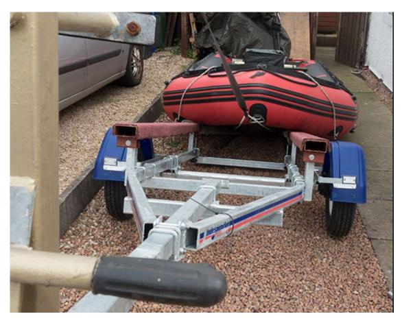
I prefer trailers with a metal beam that runs from port to starboard at the back of the trailer. Your transom should always be supported by the trailer, in case the pontoons deflates whilst in transit (which will happen on a cold winters' night!)
